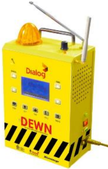
Figure 14: The DEWN Device. Source: University of Moratuwa. DEWN devices are activated by the reception of an SMS or a Cell Broadcast message.
