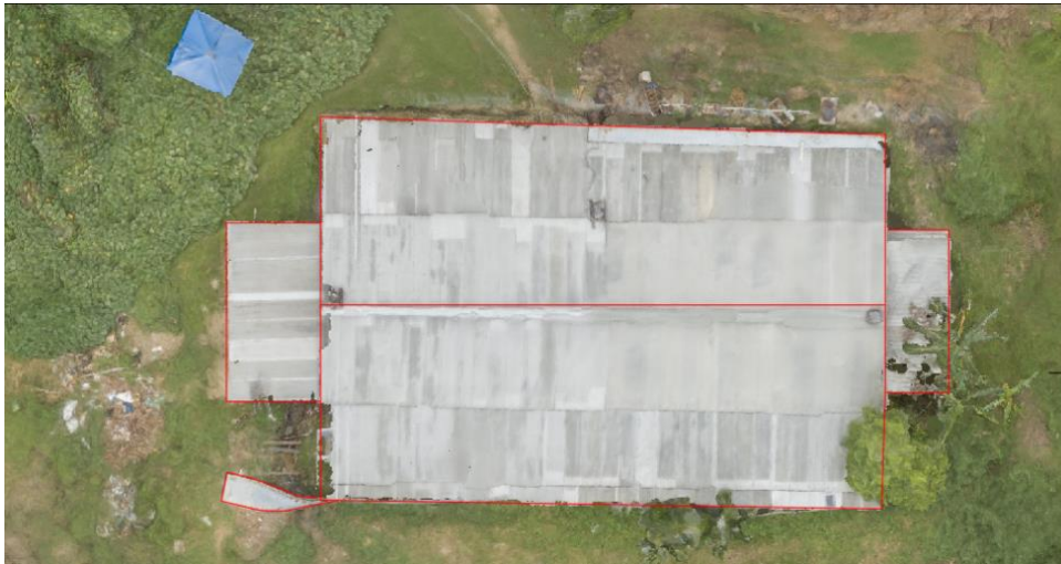
Figure 48. CAD reconstruction of farm elements (main pig house with both porches and steel foil wind barrier) from Top view orthophoto
