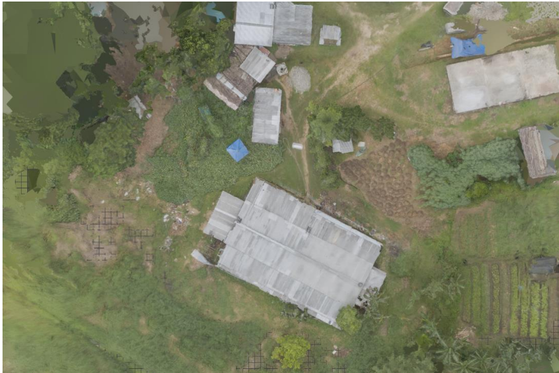
Figure 41. Orthophoto from top. The picture is now correctly oriented towards the magnetic north, and in non-perspective scale
