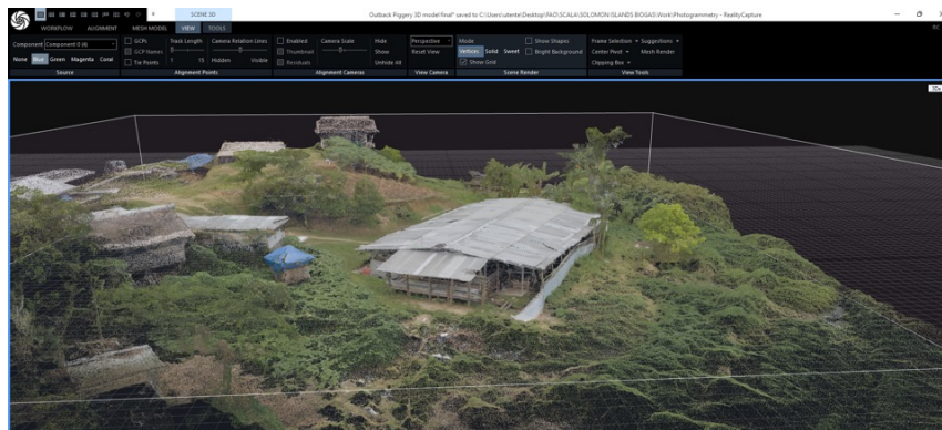
Figure 39. Above the Point Cloud with vertices is transformed into a solid 3D object that has continuous surfaces instead of individual points in space. The 3D object is then simplified to reduce its complexity and weight while retaining its characteristics and information
