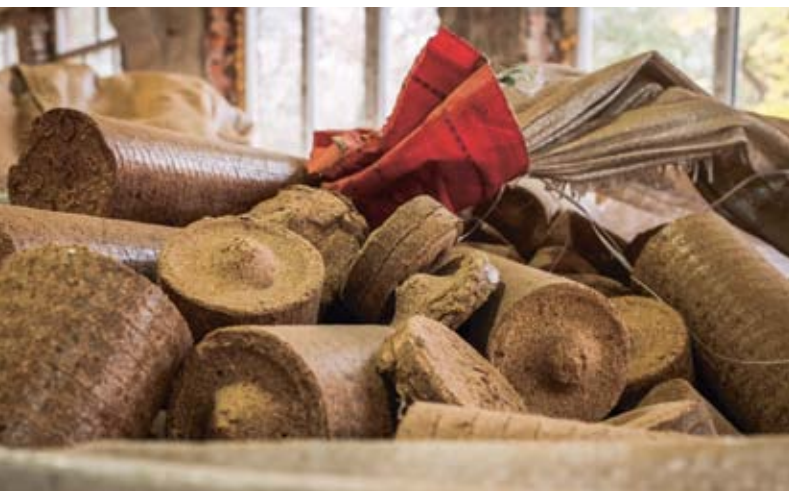
The briquettes are made from compressing wood and wood chips
